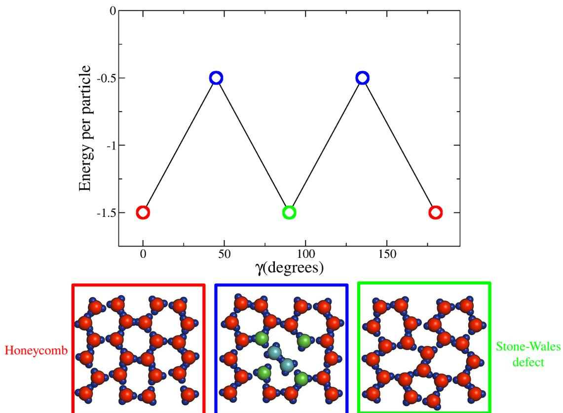
FIG. 2: Patchy model designed to reproduce the metastability of the Stone-Wales defect with respect to the honeycomb structure.
